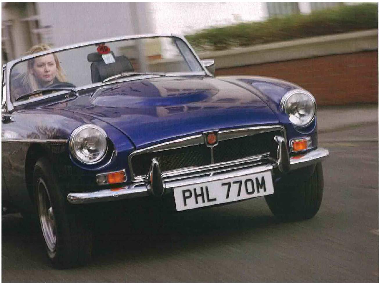
Bonnet power hump, wheelarch extensions and Wolfrace wheels – the height of Seventies fashion
