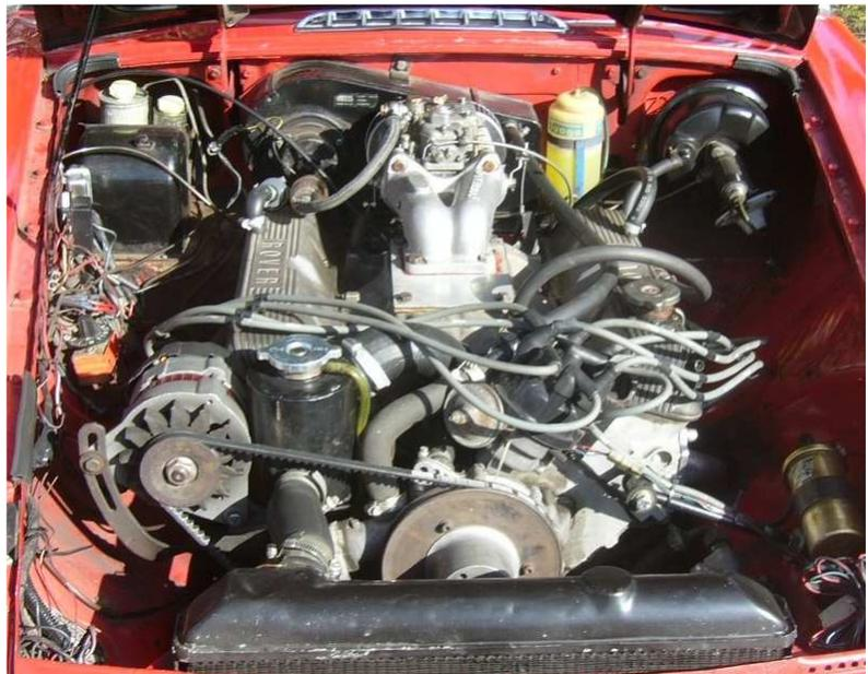
On chrome bumper cars, the firm first fits new chassis rail engine mounts and modifies the steering shaft to avoid obstruction to the V8 exhaust manifold, before removing the original radiator mountings and fitting the later type. Both the front pan and front bulkheads are then cut away and the brake light switch resisted. Having completed this first step, the engine bay is ready to take the V8 unit in the same way as the later MGB models.
