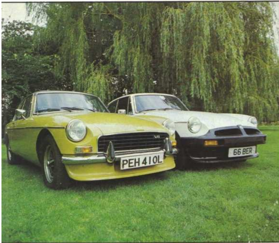
A 1.5-inch greater ride height in the late-model MGB is exaggerated by the larger rubber front bumper; even so, there is no missing the sleeker stance of the chrome-bumper car (left). The V8 nature of each version is apparent from the rear badging, but the Costello conversion adds its name to complete the picture (above)
