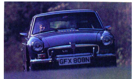
Standard factory V8, introduced in 1973, came only in GT version. V8 badging on grille, rear panel, and near side wing, plus alloy wheels are only recognition points.
