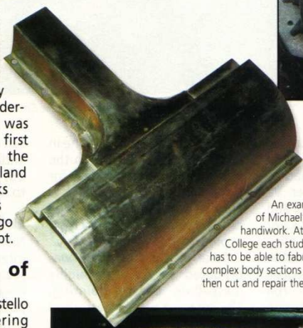
Michael made a replacement radiator header tank in stainless steel to match the original Costello steel design
