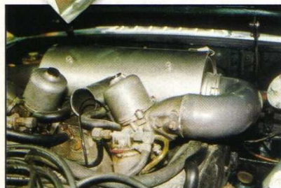
The main reason for the bulge is the original Rover mid mounted SUs with their substantial air cleaners
