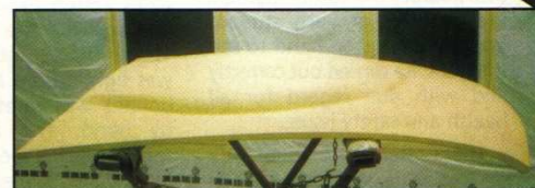
The fibreglass bonnet after repair and spraying with high build primer
